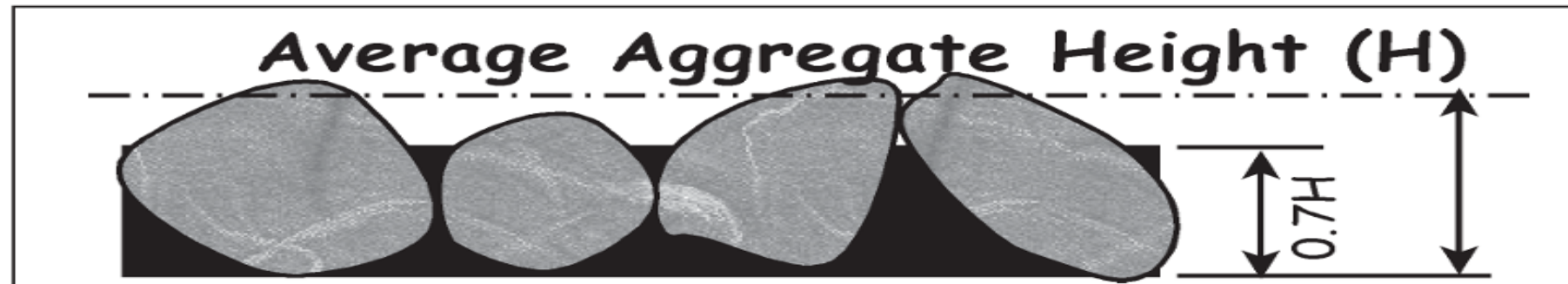
Figure 25. McLeod Design: One-Stone-Thick and Proper Embedment (70%)
