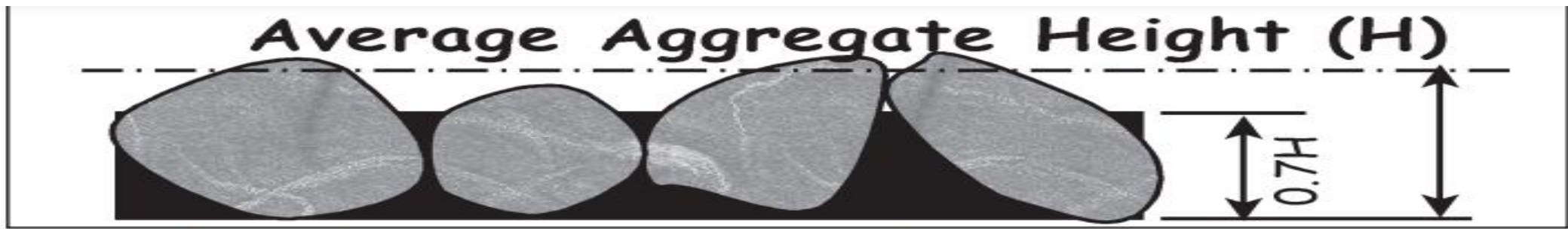
Figure 4.3. McLeod design: One-stone thick & proper embedment
